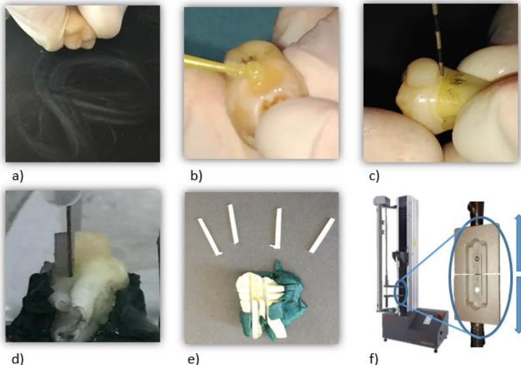
a) Flat and smooth surface on the buccal face. b) Implementing the adhesive strategy. c) Making a composite resin block. d) Sectioning the resin block with the microtome. e) Resulting specimens. f) Microtensile test in universal testing machine.
