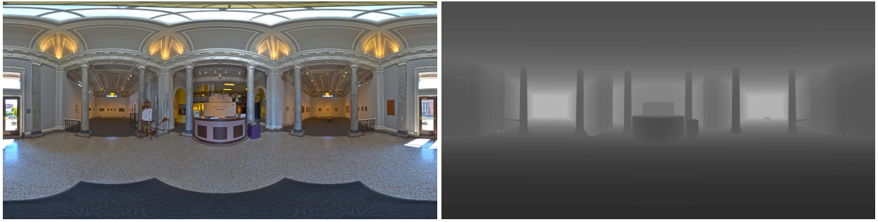
Figure 7: The left picture shows the radiance channel of the environment and the right one the depth channel used to reconstruct the light positions. Panorama courtesy of Sam Schad, www.blendedskies.com .
