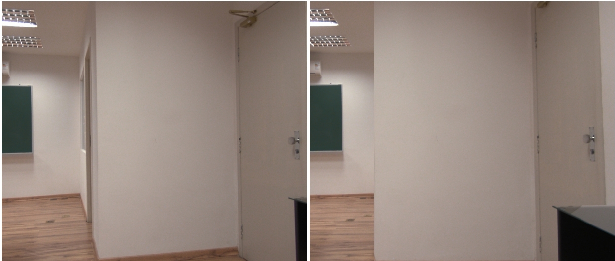
Figure 16: Detail of the camera traveling effect. A door partially visible in the left image is occluded by the wall in the right one. Left: Camera positioned where the environment was captured. Right: The camera is displaced from the environment origin.
